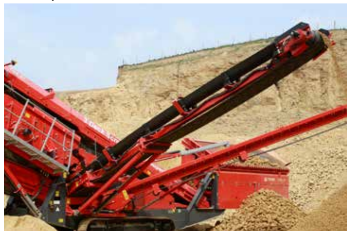
Middle Grade Conveyor
