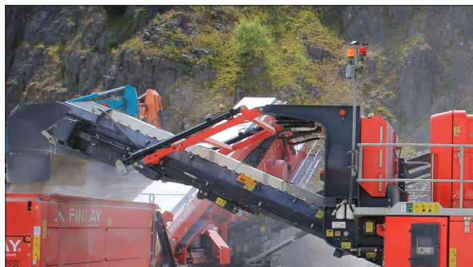
Main Conveyor - shown with optional dust covers
