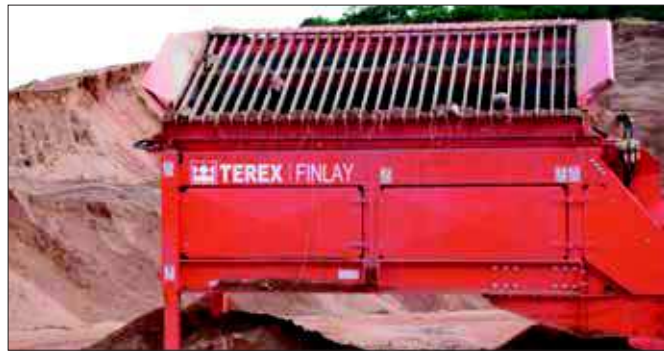
Hopper and Grid
